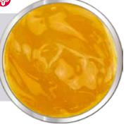
LUKOIL SIGNUM LP 00-150 can be used in roller and plain bearings of vehicles, working and production machinery. Due to its excellent pumpability it is ideally suited for central lubrication systems. The universal application area reduces the risk of mix-up and storage costs. This fluid grease is also designed for continuous operation at high pressure and in a wide temperature range. It remains at the lubricating point over a wide temperature range.
